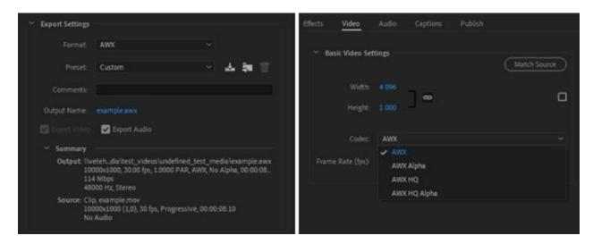
After encoding the AWX media file it is ready for playback with Analog Way Picturall Mark II media servers. Upload the file to the server with Commander UI or with Web configurator media management (see the User manual for more detailed instructions).
